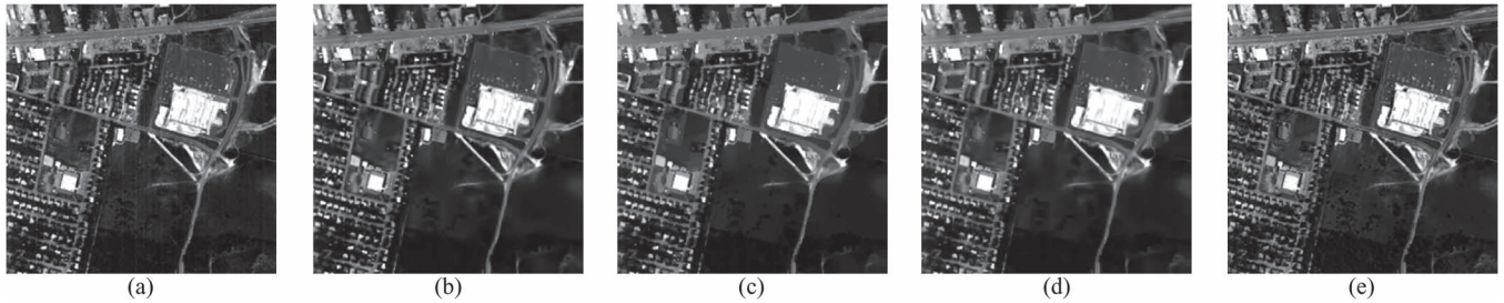
Fig. 20. Restoration results of band 2 in the real data experiment 1: (a) Original, (b) wavelet, (c) SSAHTV, (d) VBM3D, and (e) LRMR.
