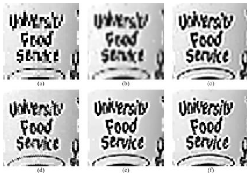
Fig. 13. Detailed regions cropped from Fig. 12. (a) LR image. (b) Bilinear interpolation. (c) Tikhonov regularization. (d) BTV regularization. (e) TV regularization. (f) SWTV regularization.
