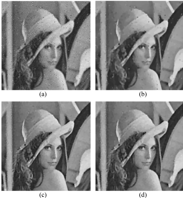
Fig. 5. Restoration results of the Lena image in the mixed noise case ( 5 \times 5 blur, standard deviation = 1.5). (a) Degraded image. Result of the (b) l_2 norm, (c) l_1 norm and (d) Proposed adaptive norm.
