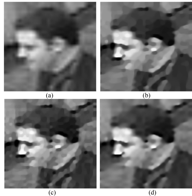
Fig. 17. Results for the compressed face sequence in the second real data experiment. (a) Original noisy image (b)–(d) Results for l_2 + TV , l_1 + TV , and the proposed method, respectively.
