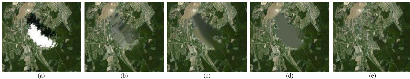
Fig. 9. Experimental results for the recovery of a cloudy image. (a) Original cloudy image. Recovered images using the following: (b) the kriging interpolation method in [23]; (c) the BSCB diffusion method in [7]; (d) the TV regularization method in [11]; and (e) Criminisi's exemplar-based method in [19].
