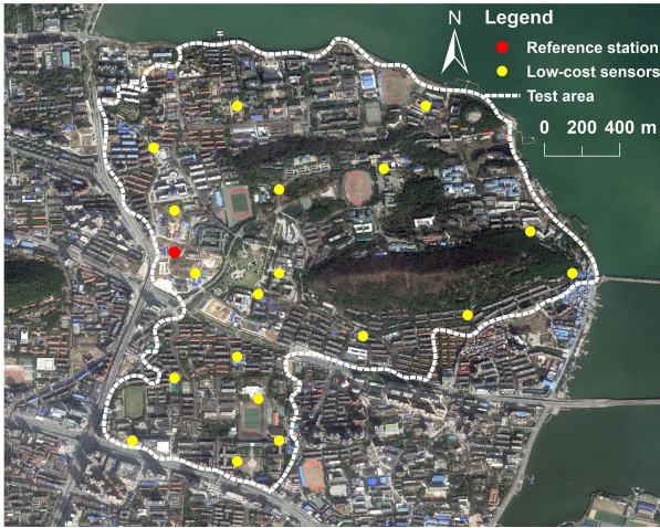
Fig. 6. Deployment of the low-cost integrated sensors at Wuhan University. (The map was obtained from Global Mapper.)
