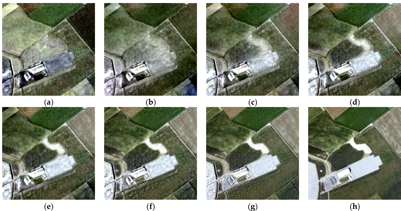
Figure 9. Fusion results of adjustability experiment in area 1. (a) IHS fusion; (b) LPSR-5; (c) LPSR-4; (d) LPSR-3; (e) LPSR-2; (f) LPSR-1; (g) LP-based fusion; (h) original HR multispectral image.
