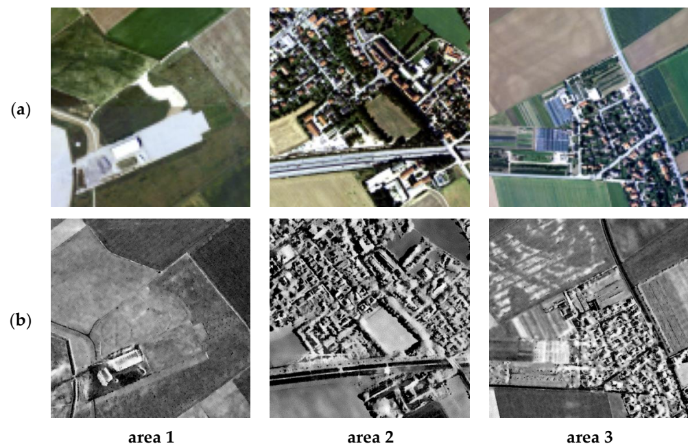
Figure 3. Multispectral and SAR images used for fusion experiments, located in the Trudering region of Munich in Germany. (a) Airborne multispectral images; (b) airborne SAR intensity images.
