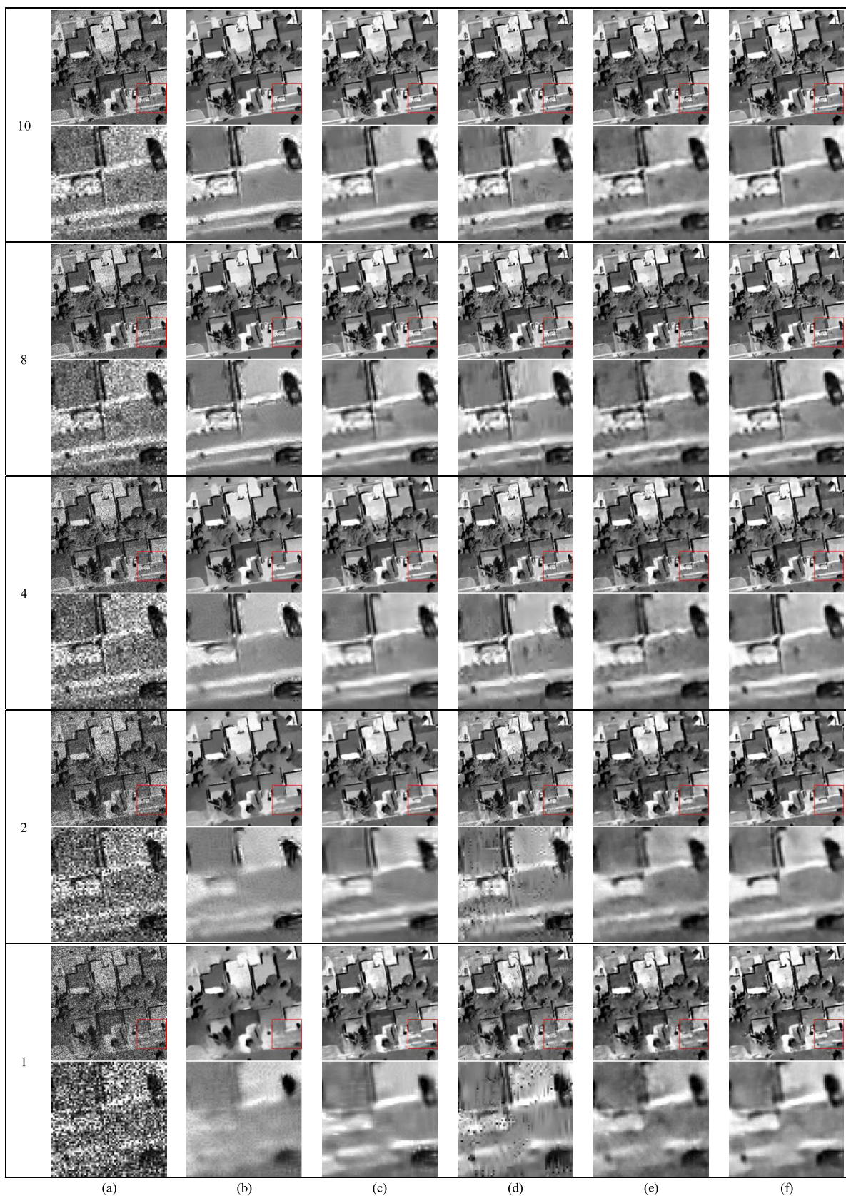
Fig. 6. Despeckled images for the medium-residential image. (a) Noisy image. (b) SAR-PPB. (c) SAR-BM3D. (d) SAR-POTDF. (e) SAR-DRN. (f) Proposed method.
