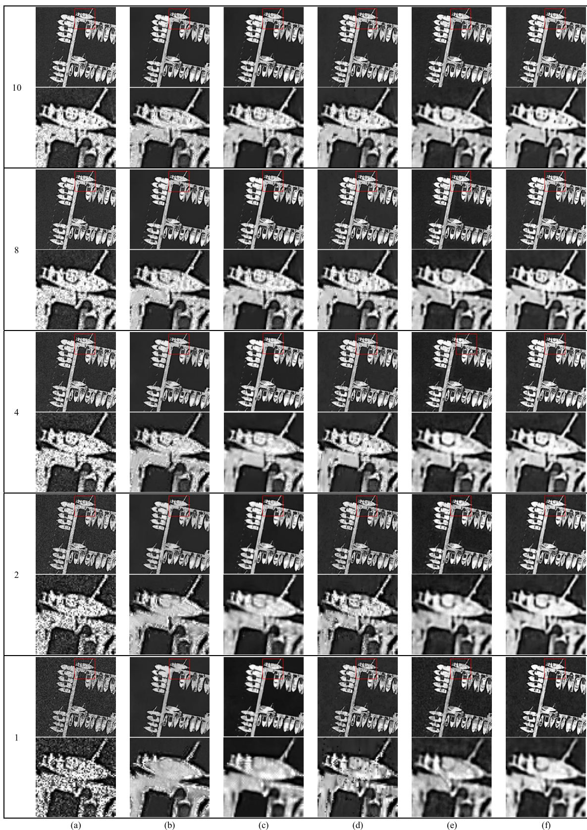
Fig. 5. Despeckled images for the harbor image. (a) Noisy image. (b) SAR-PPB. (c) SAR-BM3D. (d) SAR-POTDF. (e) SAR-DRN. (f) Proposed method.
