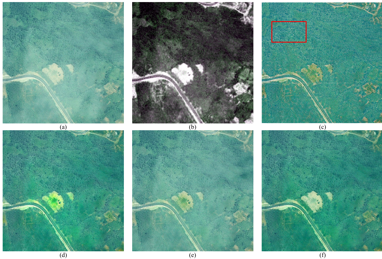
Fig. 7. Haze removal results for a forest image. (a) Hazy image. (b) HOT. (c) FVR. (d) TDCP. (e) DSP. (f) Proposed method.
