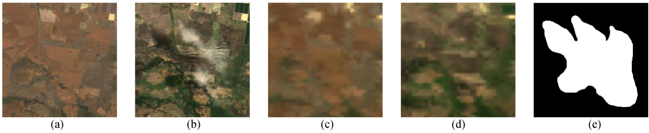
Fig. 7. Data with observed clouds used for the algorithm testing (with the red, green, and blue bands as RGB). (a)–(b) Landsat images of October 25, 2004, and January 29, 2005, respectively. (c)–(d) Resampled MODIS images corresponding to (a) and (b). (e) Cloud and cloud shadow mask of (b) obtained by visual interpretation.
