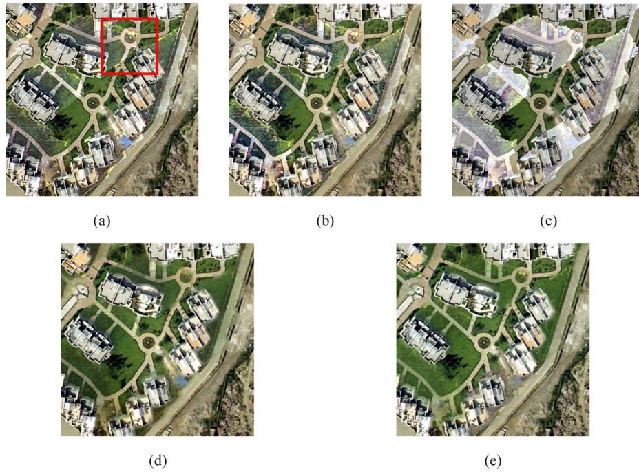
Fig. 4. Shadow removal results for image #1. (a) Result of the LCC method. (b) Result of the HMC method. (c) Result of the SMIT method. (d) Result of the SANL method. (e) Result of the proposed method.
