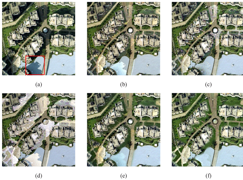
Fig. 8. Image #3 and its shadow removal results. (a) Original image with shadows. (b) Result of the LCC method. (c) Result of the HMC method. (d) Result of the SMIT method. (e) Result of the SANL method. (f) Result of the proposed method.
