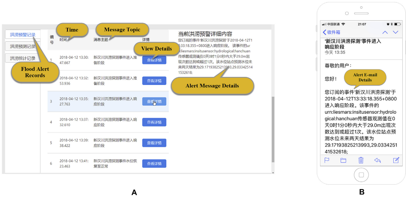
Fig. 14. The flood alert record interface and alert E-mail of the PFD&S prototype. (a) The flood alert records interface; (b) The flood alert E-mail.
