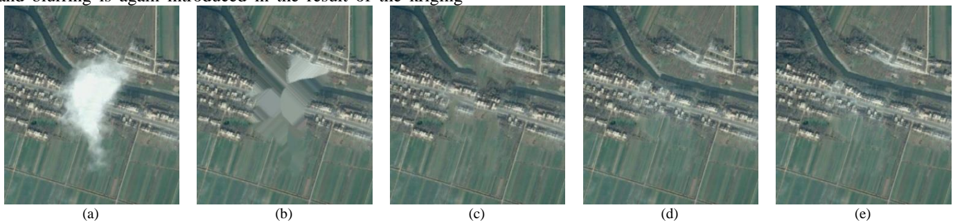
Fig. 3. The first real data experiment. (a) Original cloud-contaminated GeoEye-1 image. Cloud removal results by the following methods: (b) kriging interpolation method; (c) Content-Aware Fill method; (d) He et al. 's method; and (e) the proposed method.
