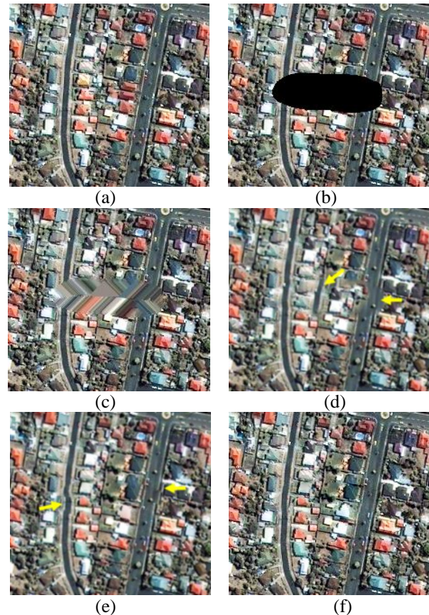
Fig. 2. Simulated data experiment. (a) Original IKONOS image. (b) Simulated image with missing region. Reconstructed images by the following methods: (c) kriging interpolation method; (d) Content-Aware Fill method; (e) He et al. 's method; and (f) the proposed method.
