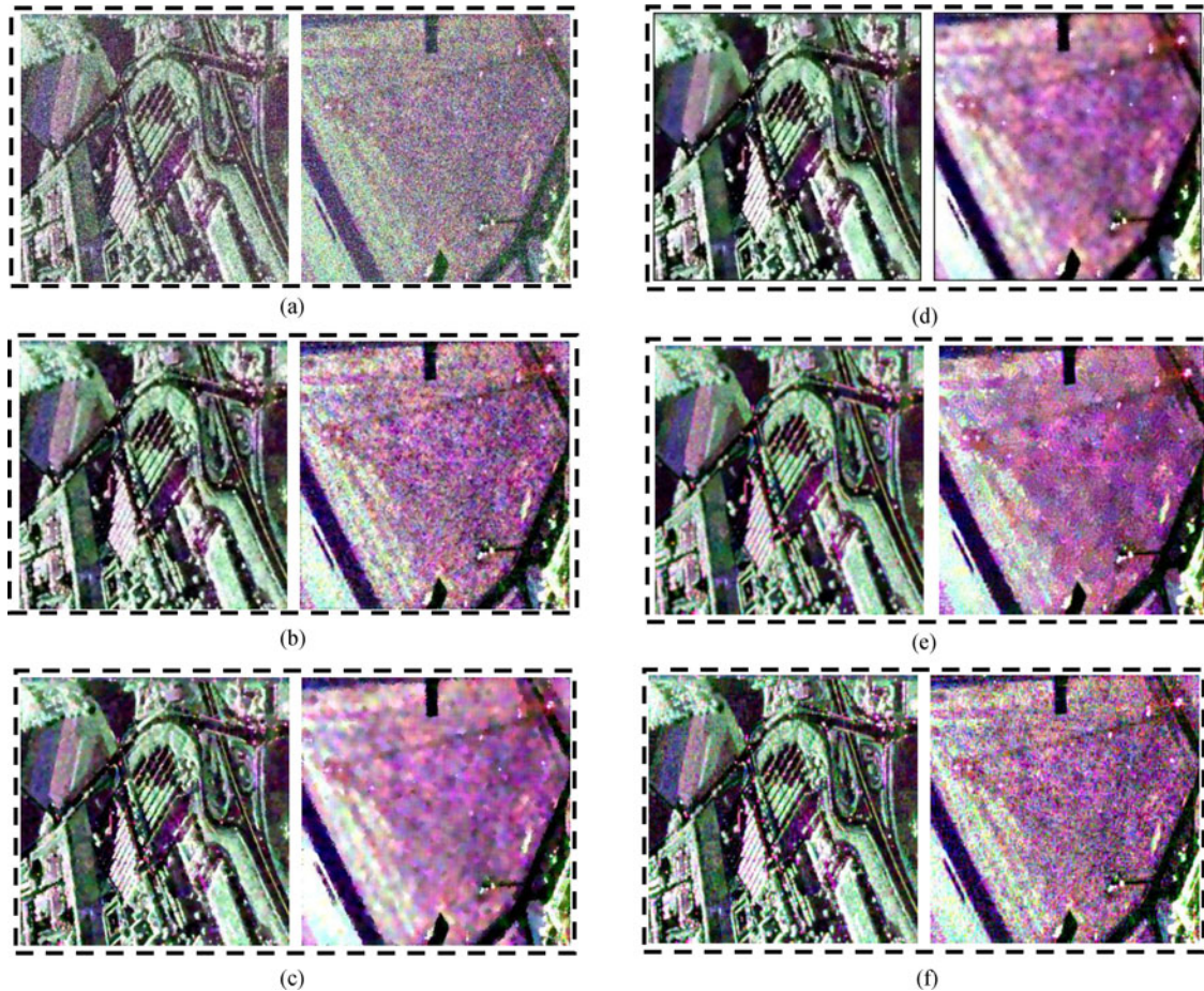
Fig. 9. Filtering results on two subimages of the Oberpfaffenhofen dataset. (a) Speckled data. (b)–(f) Filtering results of the extended sigma filter ( \xi = 0.8 , w_1 = 7 \times 7 ), the AIR-PAD filter ( T = 15 ), the pretest NLM filter ( k = 20 , w_2 = 3 \times 3 ), the PolSAR NLTv method ( r = 5 , w_2 = 3 \times 3 ), and the PolSAR SSC method, respectively.
