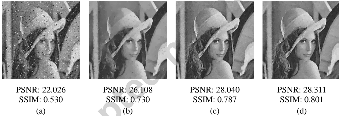
Fig. 6. The SR reconstruction results of the Lena image by (a) bilinear interpolation, and (b) MAP with l_2 -norm fidelity, (c) l_1 -norm fidelity, and (e) l_p -norm fidelity, with p=1.3 .
