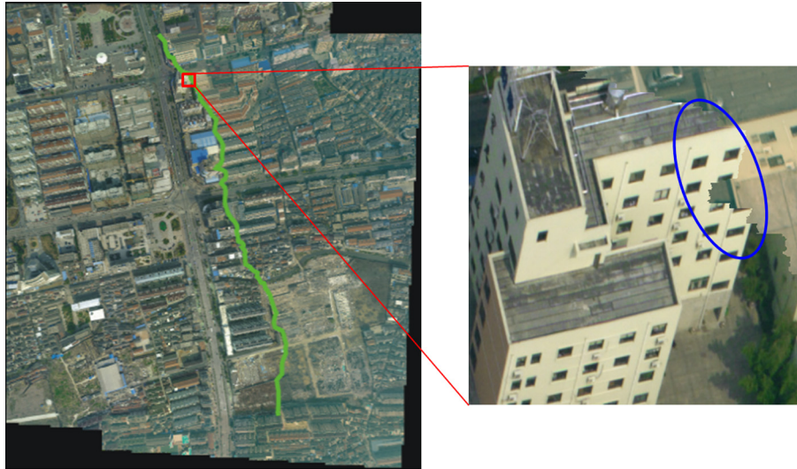
Fig. 15. A poor seamline, with the seamline going through the building. The left image is the same as Fig. 14(b).
