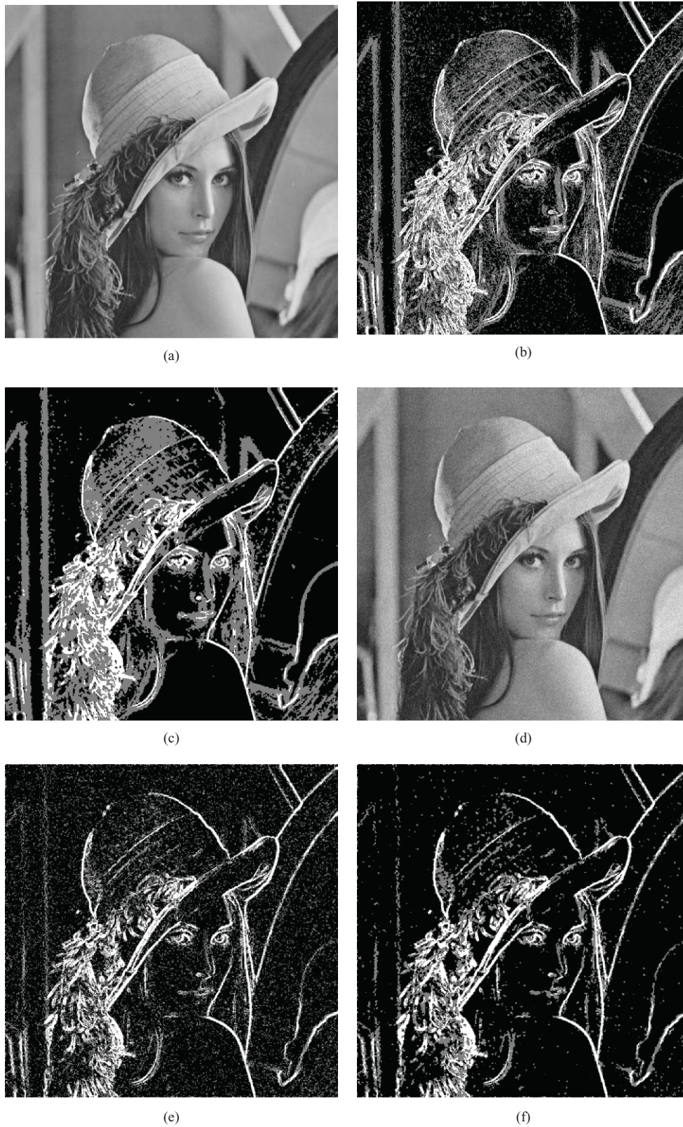
Fig. 2 Region map for Lena image: (a) Original Lena image, (b) region map corresponding to (a) ( \sigma = 0.05 , \rho = 0.1 ), (c) region map corresponding to (a) processed by majority filtering ( \sigma = 0.05 , \rho = 0.1 ), (d) noisy lena image, (e) region map corresponding to (d) ( \sigma = 0.3 , \rho = 0.8 ), and (f) region map corresponding to (d) processed by majority filtering ( \sigma = 0.3 , \rho = 0.8 ).
