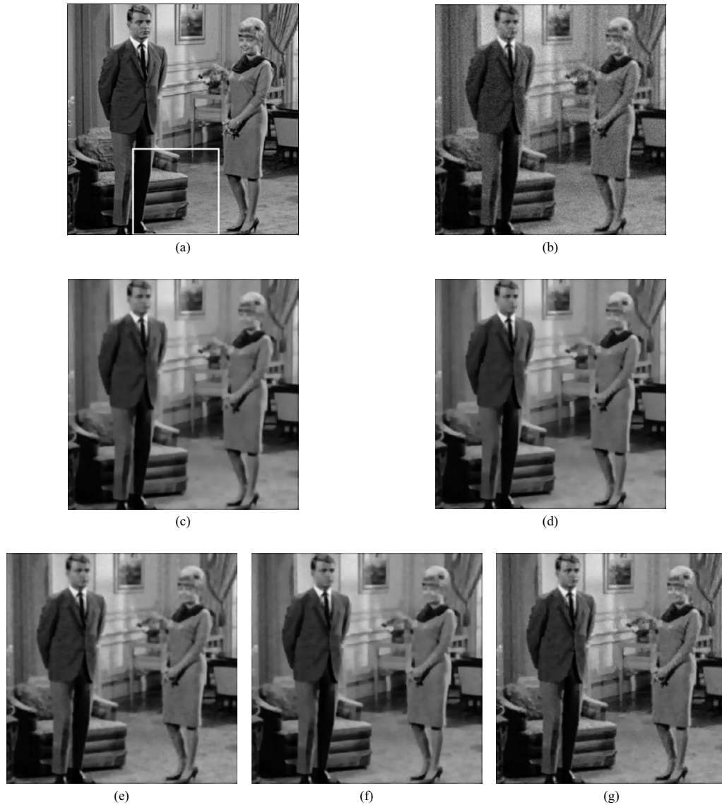
Fig. 10 Enhanced images for Couple image: (a) Original image with 8-bit gray levels; (b) Gaussianly blurred image ( \sigma=1 ), contaminated by zero-mean Gaussian noise with 50; (c) CLMC anisotropic diffusion ( \rho=0.05 ); (d) MB anisotropic diffusion ( \rho=0.05 ); (e) GSZ FAB diffusion ( k_f=0.2 \cdot \text{MAG} , k_b=0.4 \cdot \text{MAG} , \alpha=0.2 ); (f) LVCFAB diffusion ( k_f=50 , k_b=200 , \beta_1=0.2 , \beta_2=0.02 , \rho=0.2 , \alpha=0.2 ); and (g) TFAB diffusion ( \beta=0.006 , \gamma=8 , \xi=2 ) (15 iterations).
