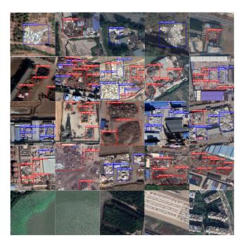
Fig. 4. Results of the proposed LKN-ME method with the DSWD test dataset. The first row shows images with single solid waste objects. The second to fourth row show images containing multiple solid waste objects. The fifth row shows images with objects that are similar to solid wastes.
