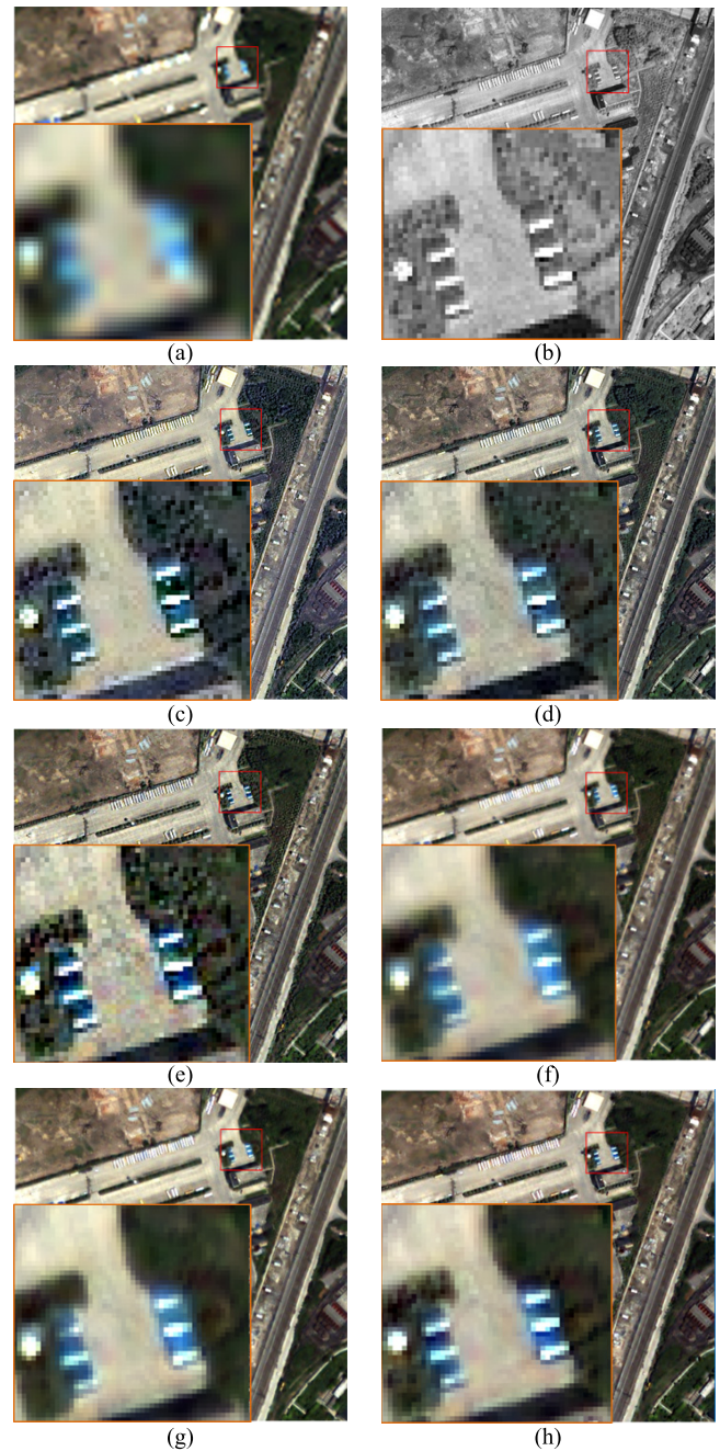
Fig. 10. Real-data fusion results of the IKONOS image. (a) LR-MS image. (b) HR-PAN image. (c) AIHS. (d) MTF-GLP-HPM. (e) TSSC. (f) DNCNN. (g) DRPNN. (h) Proposed method.
