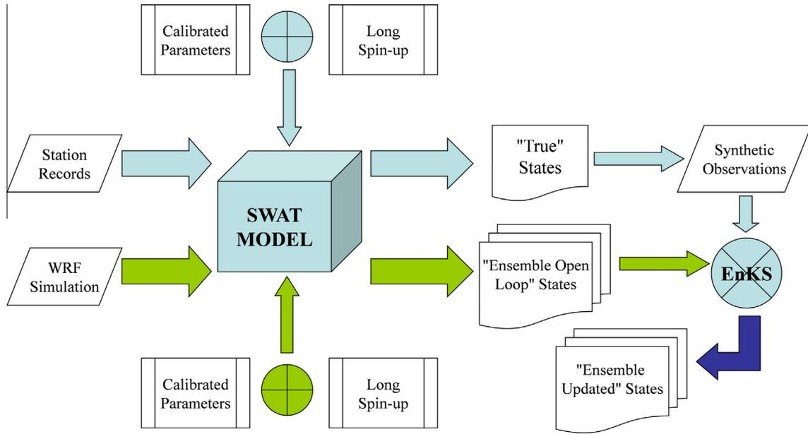
Fig. 2. Flowchart of the OSSE experiment.
